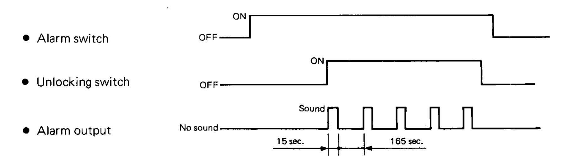
During the alarm time, the sound continues for 15 seconds on average (about 10–20 seconds), followed by 165 seconds on average (about 110–210 seconds) of soundless alarm, and this process is repeated 5 times on average (3–7 times). — Snooze alarm.
