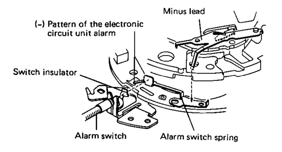
One end of the minus lead is connected to the power cell connector (-). The other end of the minus lead is connected to the alarm switch spring.
