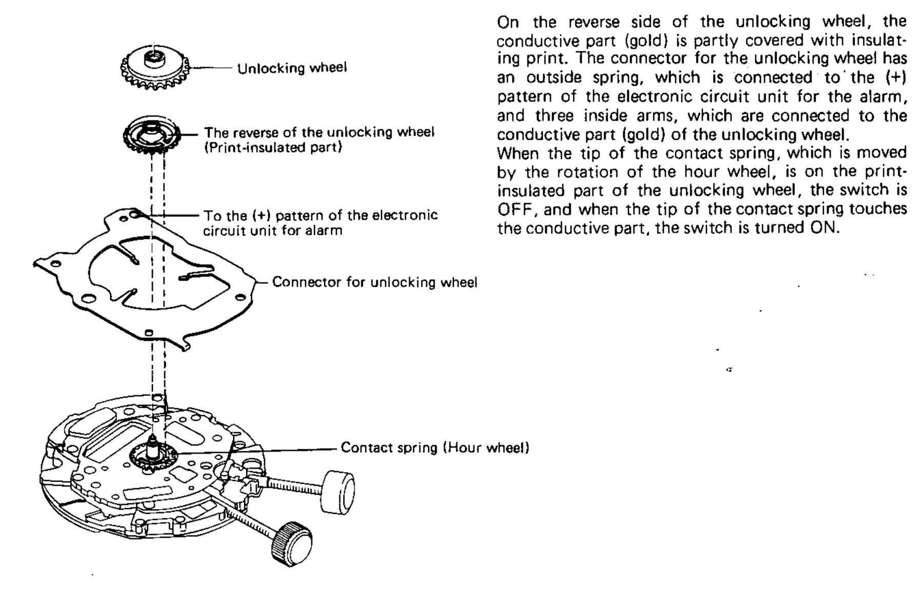
The alarm begins to sound when both switches, 1 and 2 are ON.
